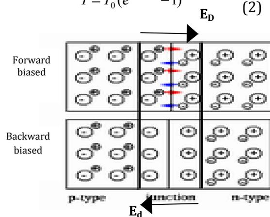
Figure 1. A p-n junction diode.
