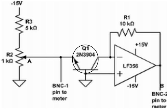
**Figure 2: Circuit used to determine Boltzmann's constant.**
